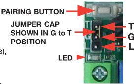
**T:** Toggle (Alternate Action) **L:** Interlocked
